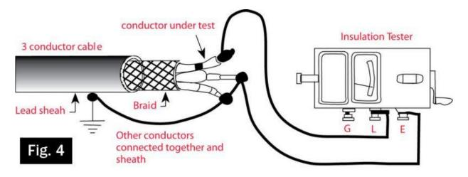
Note that IR is temperature sensitive. When the temperature goes up, IR goes down, and vice versa. Therefore, to compare new readings with previous readings, you need to correct the readings to some base temperature. Usually, 20°C or 40°C are used as comparison temperatures; tables are available for any correction. However, a common rule of thumb is that IR changes by a factor of two for each 10°C change.
