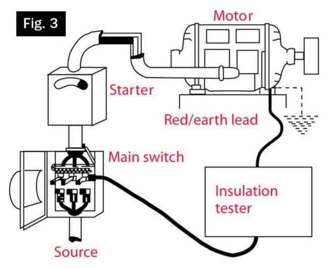
This is the simplest of the tests. After the required connections are made, you apply the test voltage for a period of one min. (The one-min interval is an industry practice that allows everyone to take the reading at the same time. In this way, comparison of readings will be of value because, although taken by different people, the test methods are consistent.) During this interval, the resistance should drop or remain relatively steady.
